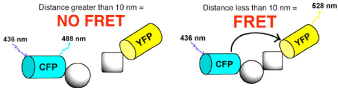
**Figure 7.** FRET depends on the close proximity of a donor and acceptor pair of fluorescent molecules in which the emission spectrum of the donor overlaps the excitation spectrum of the acceptor. Because these molecules must be within 10 nm for FRET to occur, the spatial resolution of the microscope is significantly improved.
