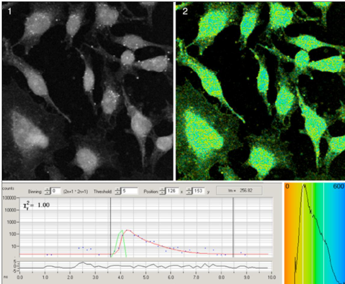
**Figure 6.** A nuclear protein has been labeled with CFP and imaged using a multiphoton FLIM system. It is helpful to compare a fluorescence intensity image (1) with the fluorescence lifetime map (2) in order to compare lifetimes among different regions of the sample. In this case, the lifetime for CFP is approximately 500 picoseconds.
